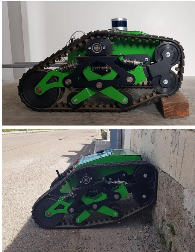
Fig. 12: Experimental validation using the tracked robot Polibot: obstacle traverse (top), upward wall navigation (bottom)
